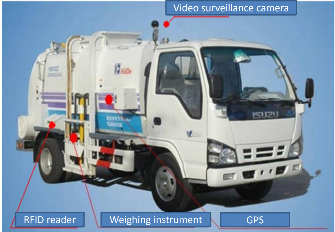
FIGURE 1. TRUCKS INSTRUMENTED WITH RFID READER, GPS, WEIGHING INSTRUMENT, AND VIDEO SURVEILLANCE CAMERAS IN SUZHOU
